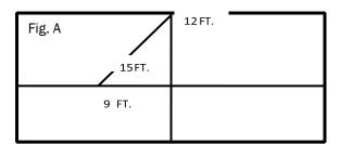
To verify that the working lines are square with each other measure 12' from the center point up the vertical length and make a mark. On the same horizontal quadrant line measure 9' across the width and make a mark, the diagonal measurement between the two marks should be exactly 15' if your lines are square. If your measurement is not 15' adjust your lines accordingly (see fig. A).
