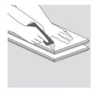
2) Remove the tongue, on the long side of the planks that face the wall on your first row. This is to ensure that the decorative surface of the flooring is well under the finished trim when installed. Use a utility knife to score through the tongue several times until it easily snaps off. Seal the cut edges with a silicone sealant.
