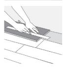
9) To fit the last row, lay a plank on top of the previous row. With the tongue to the wall, lay another plank upside down on the one to be measured and use it as a straight edge. Don't forget to allow room for the expansion spacers. Cut the plank and attach into position.
