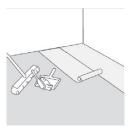
1) For planks without pre-attached cushion, install foam underlay. Run the foam underlay in the same direction as the flooring panels. Underlay should be butted side by side with no overlap. Tape seams together. Do not install an additional underlayment under planks with pre-attached cushion.
