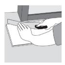
11) You can undercut door frames by turning a panel upside down and using a handsaw to cut away the necessary height so that panels slide easily under the frames.
