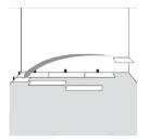
6) Begin the next row with the off-cut piece from the previous row to stagger the pattern. Pieces should be a minimum of 8" (20 cm) long and joint offset in adjoining rows should be at least 16 (40 cm).
